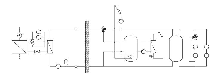
The controller is able to manage up to **two zones in heating** (one by means of a mixed circuit and the other by means of a direct circuit) and **one zone in cooling** (by means of a mixed circuit).
