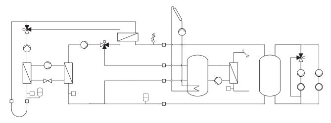
The controller is able to manage up to **two zones in heating** (one by means of a mixed circuit and the other by means of a direct circuit) and **one zone in cooling** (by means of a mixed circuit).
